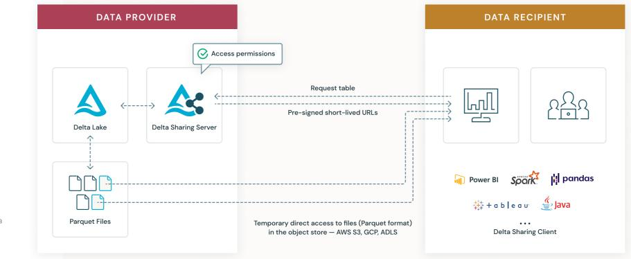
Figure 7: How Delta Sharing works connecting data providers and data recipients
