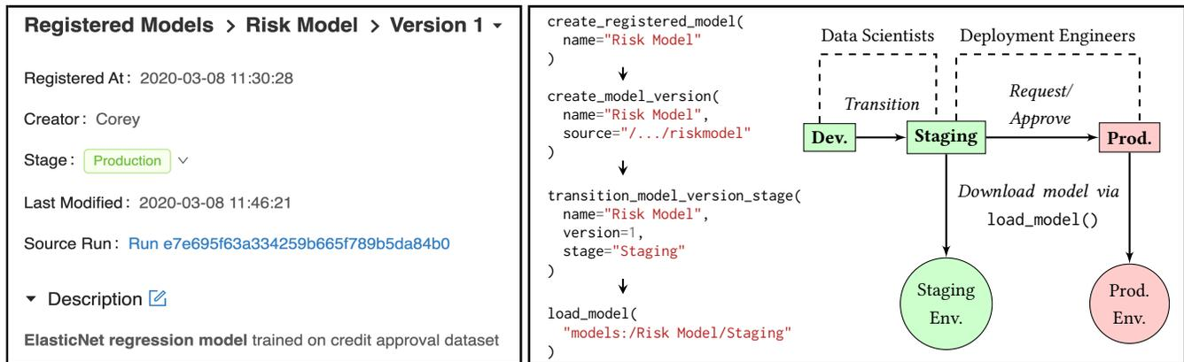
**Figure 1: Left: The Model Registry UI displays author and lineage information for each model; users can transition model versions through predefined lifecycle stages and add markdown descriptions. Right: A diagram depicting an example collaborative Model Registry workflow where models are deployed to staging and production environments; a sequence of API calls for the "Data Scientists" portion of the workflow is also displayed.**
